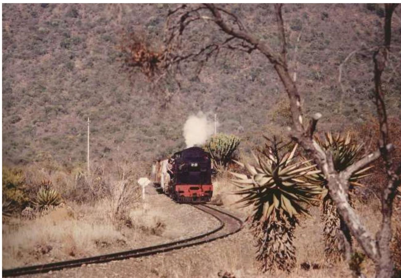
***Spectacular scenery provides a wonderful backdrop for a Narrow Gauge Garratt locomotive hauling a mixed train of freight and passenger cars. But note how the line twists and turns as it climbs up from the valley. No wonder the locomotives required two water stops when travelling away from Estcourt.***
